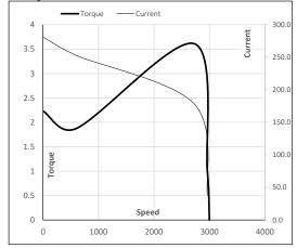
Motor Speed Torque Data P-Up BD Rated NL LR Load Point Speed r/min 0 600 2725 2963 3000 Current А 280.9 252.8 178.4 38.0 12.6 Torque ри 2.2 1.9 3.6 1 0
