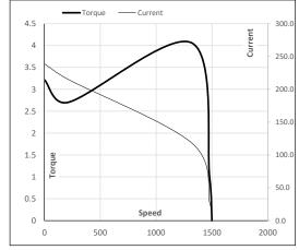
P-Up BD Rated NL LR Load Point Speed r/min 0 214 1321 1479 1500 Current А 239.0 215.1 118.2 28.1 11.0 Torque pu 3.2 2.7 4.1 1 0
