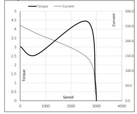
Motor Speed Torque Data P-Up BD Rated NL LR Load Point Speed r/min 0 600 2640 2961 3000 Current А 252.5 227.3 144.1 27.4 9.2 Torque ри 3.0 2.5 4.4 1 0
