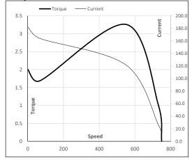
Motor Speed Torque Data P-Up BD Rated NL LR Load Point Speed r/min 0 68 551 732 750 Current А 182.3 164.0 121.5 26.0 13.9 Torque ри 2.0 1.7 3.3 1 0
