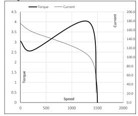
Motor Speed Torque Data P-Up BD Rated NL LR Load Point Speed r/min 0 214 1318 1479 1500 Current 174.4 157.0 104.3 21.3 10.9 А Torque pu 3.1 2.6 4.0 1 0
