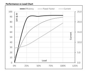
Motor Speed Torque Data LR P-Up BD Rated NL Load Point 600 2650 2960 3000 0 Speed r/min Current Α 170.8 153.7 105.6 19.4 7.1 Torque pu
