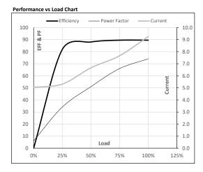
Motor Speed Torque Data LR P-Up BD Rated NL Load Point 91 828 978 1000 0 Speed r/min Current Α 61.1 55.0 35.3 9.3 5.0 Torque 0 pu
