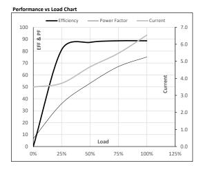
Motor Speed Torque Data LR P-Up BD Rated NL Load Point 0 91 837 976 1000 Speed r/min 6.5 Current Α 39.9 35.9 23.3 3.5 Torque 0 pu
