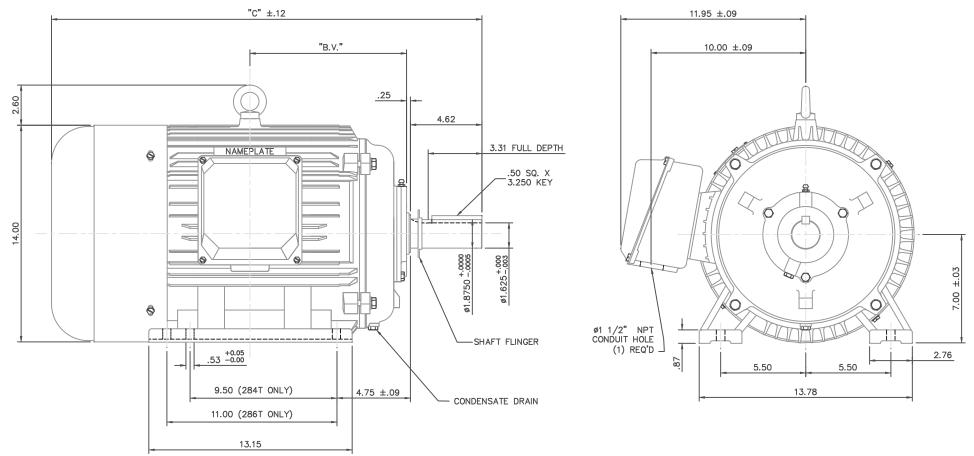
NOTE: 286T HAS 6 MTG. HOLES, USING 284T AND 286T LOCATIONS
