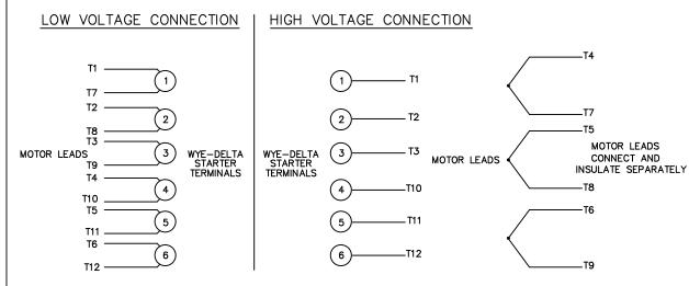
REFER TO THE WYE-DELTA STARTER CONNECTION INSTRUCTIONS FOR PROPER CONNECTION OF POWER LINES TO STARTER.
