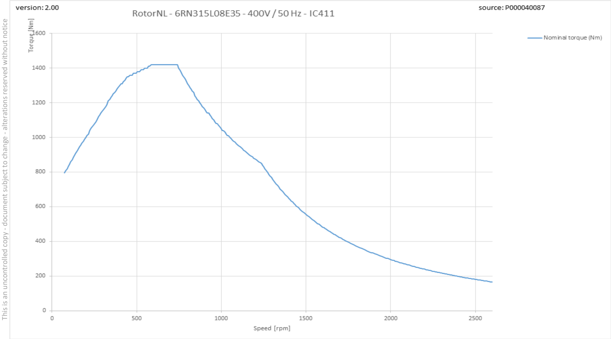
Torque versus Speed curve with variable frequency drive
