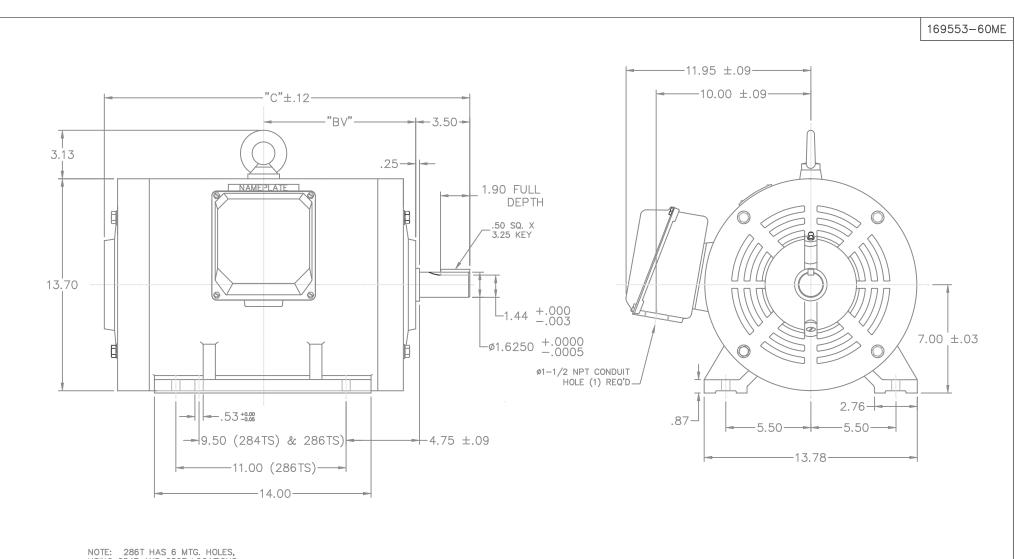
NOTE: 286T HAS 6 MTG. HOLES, USING 254T AND 256T LOCATIONS
