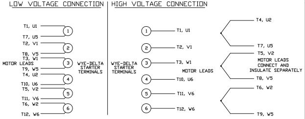
REFER TO THE WYE-DELTA STARTER CONNECTION INSTRUCTIONS FOR PROPER CONNECTION OF POWER LINES TO STARTER.
