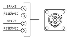
4 PIN CONNECTOR (BRAKE WHEN SPECIFIED)
