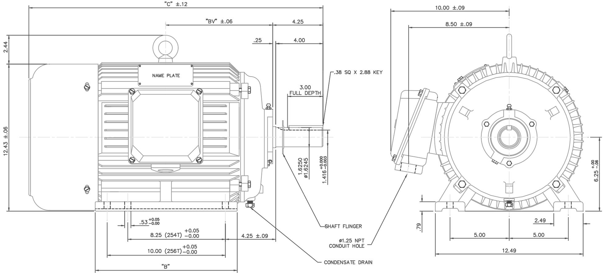
NOTE: 256T HAS 6 MTG. HOLES, USING BOTH 254T AND 256T "2F" LOCATIONS.
