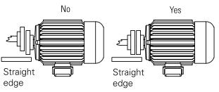
Excessive angular displacement must also be prevented. The recommended method to achieve correct angular alignment is shown below.
