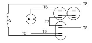
ROTATION JOIN & FACING L2 L1 INSULATE LEAD END P1 T4,T5 T1,T8 C.C.W. C.W. T4,T8 T1,T5 Ρ1
