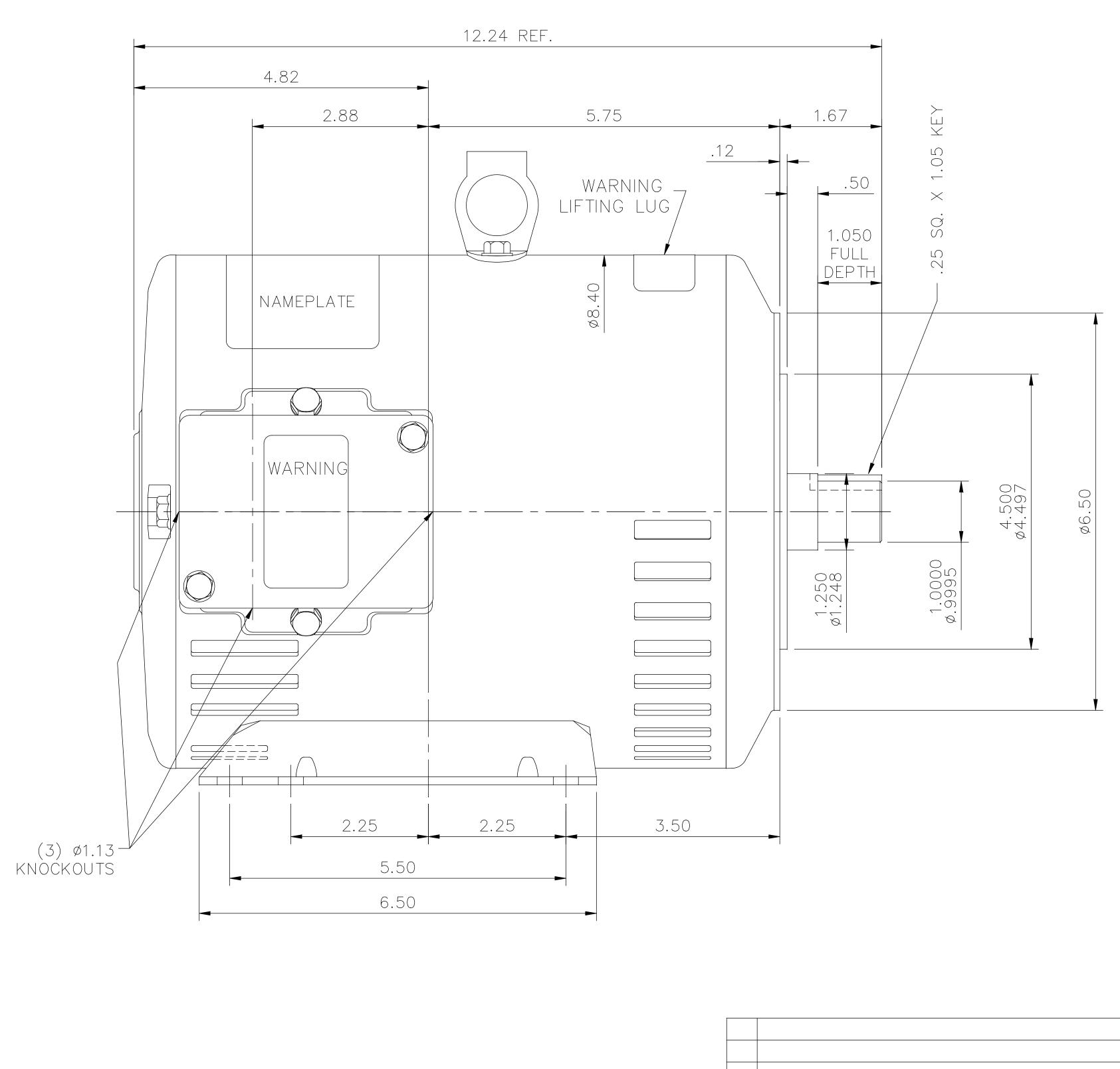
MAXIMUM FACE RUNOUT TO BE .004 T.I.R. MAXIMUM PILOT ECCENTRICITY TO BE .004 T.I.R. PERMISSIBLE SHAFT RUNOUT TO BE .002 T.I.R.
