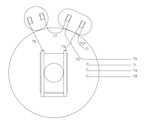
LINE LEADS \_\_\_\_ T1 – T8 T6 T7 T5 Т9 T5 ROTATION FACING L1 L2 LEAD END T4,T5 C.C.W. T1,T8 C.W. T1,T5 T4,T8
