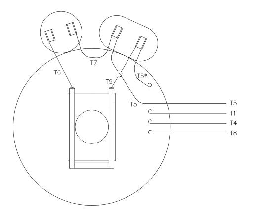
LINE LEADS – T8 T6 T7 T5 Т9 T5 ROTATION FACING L2 L1 LEAD END T4,T5 C.C.W. T1,T8 C.W. T4,T8 T1,T5
