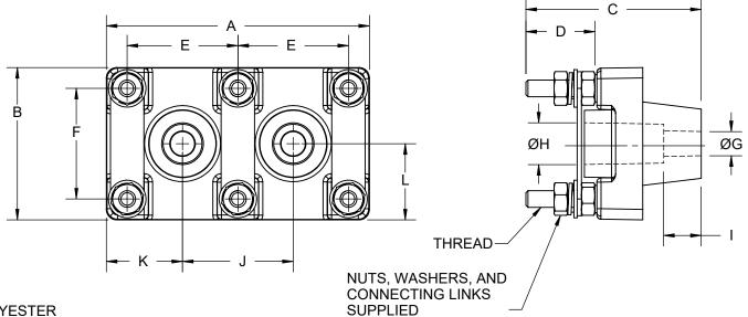
MATERIAL: BASE- THERMOSET POLYESTER STUDS AND HARDWARE- PLATED STEEL LINK- NICKEL PLATED COPPER
